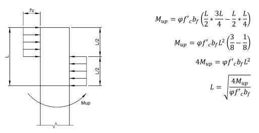
Figure 10-1: Pile Fixity
